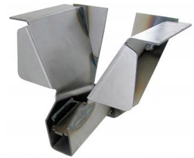
Rear jacking point (each) Bus until 7.1967
