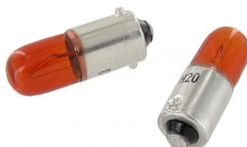
Turn indicator bulb 12V amber (Per Pair) Type: bayonet, Base: BA9s, Color: amber (orange), voltsage: 12V, Power: 4 Watt
