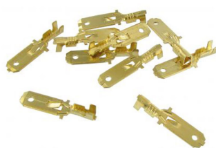
Uninsulated male spade connectors with locking barb (10 pieces) Spade connector size: 6.3mm, Material thickness: 0.8mm, Wire thickness: 0.5 - 1.0mm 2
