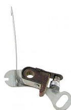
Ignition points (Garbe-Lahmeyer distributors)
