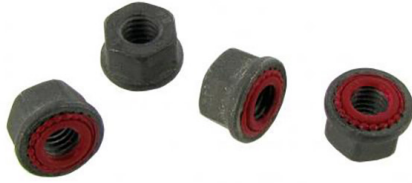
Oil pump cover nuts with seal ring (4 pieces) Type-1 engines 1200cc until 1967 (D 0 230 000), 1300cc until 1967 (E 0 013 650 and F 1 225 017), 1500cc until 1967 (L 0 018 099 and H 0 822 051), Type-3 engines 1500cc until 1967 (K 0 090 195), 1600cc until 1967 (T 0 445 097)
