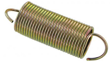
Carburetor throttle return spring Solex 28 PICT-2, 30 PICT-1, 30 PICT-2, 30 PICT-3, 31 PICT-3, 31 PICT-4, 34 PICT-3, 34 PICT-4, Brosol H30/31 PICT (#2141), Paruzzi and Solex reproductions 34 PICT-3 (#4425 and #2142)
