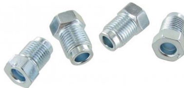
Brake line fittings (4 pieces) Thread size: M10 X 1.0, Inner size: 5.15mm, Wrench size: 11mm
