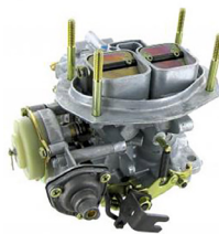
32/36 DFEV Weber carburetor Main jet: 1.30 and 1.40, Air jet: 160 and 165, Idle jet: 50 and 60, Venturi: 26 and 27mm
