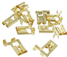
Uninsulated right angled female spade connectors with locking barb (10 pieces) Spade connector size: 7.8mm, Material thickness: 0.8mm, Wire thickness: 2.5mm 2
