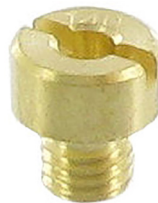
Gicleur de réglage essence Solex (the models of Solex VHS, 26 VEIS, 30 PICT, 31 PICT, 32/34 PDSIT, Solex 34 PICT, 32/34 PDSIT, Solex 35, Solex 40/44/49/24/47 PDSI, 34, HBS 32/34/36/38/40/42/44/46/48, 34 PICT 34, Paruzzi Reproducties Reproduction, 30 PICT-3, 34 PICT-3
