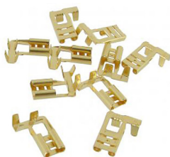
Uninsulated right angled female spade connectors without locking barb (10 pieces) Spade connector size: 6.3mm, Material thickness: 0.8mm, Wire thickness: 1.0-2.5mm 2
