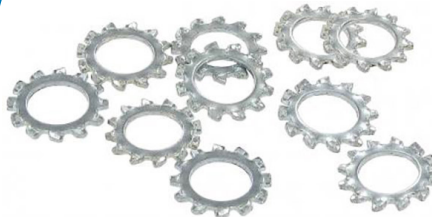
External serrated lock washers M6 (10 pieces) Inner diameter: 6,4mm, Outer diameter: 11mm, Height: 2.1mm, Material: Galvanized steel
